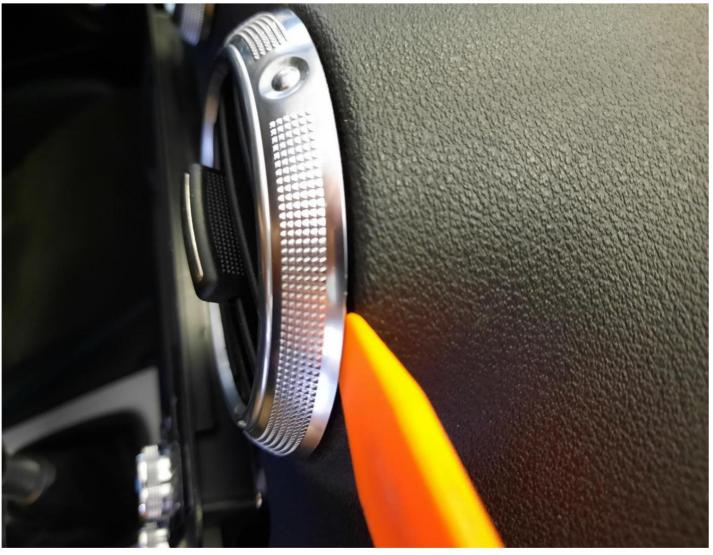
Medicate the handles with your hand and move alternately up-down, left-right pulling the airflow towards you all the time. Do the same with the second one.
